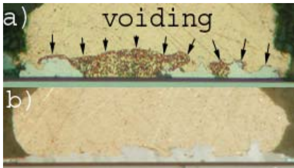
Figure 13. Cross section of wire bonds after 700 hrs. aging in air (a) and in vacuum (b). Note that extensive voiding in Au/Al intermetallic layers were observed only in the parts aged in air.
